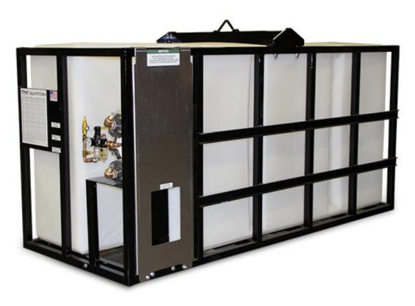
Now the task of handling fluids regardless of location, can be done easily and efficiently. The Stellar portable fluid skid is a 400-gallon poly tank with a built-in air agitator and steel tubing frame with a lifting eyelet, for ease of removal. This system also includes an anti-freeze dispenser, moisture separator, regulator, hose, ejector and fluid pumping system.
